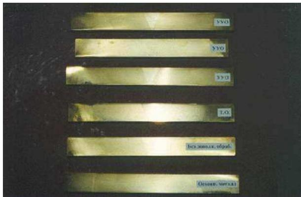
Fig. 5 Welded joints having no defects
