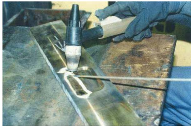
Fig. 7 Weld deposition process
