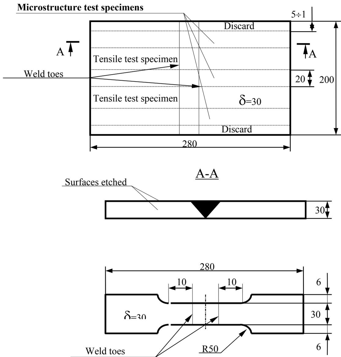
Fig. 2 Butt welded plate and tensile test specimen
