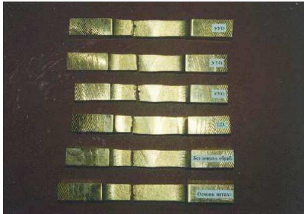
Fig. 4 Failure mode of welded specimens
