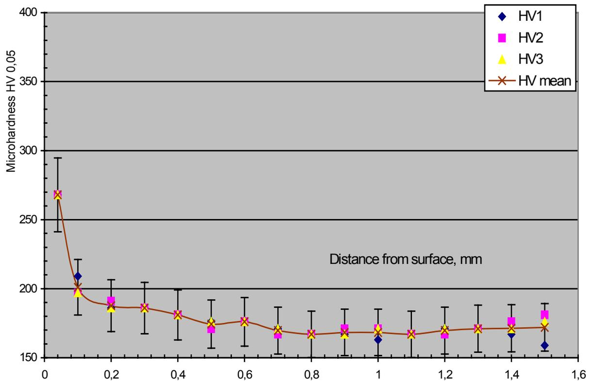
Fig. 29 Microhardness (HV 0,05 mean) of base metal after various treatments
