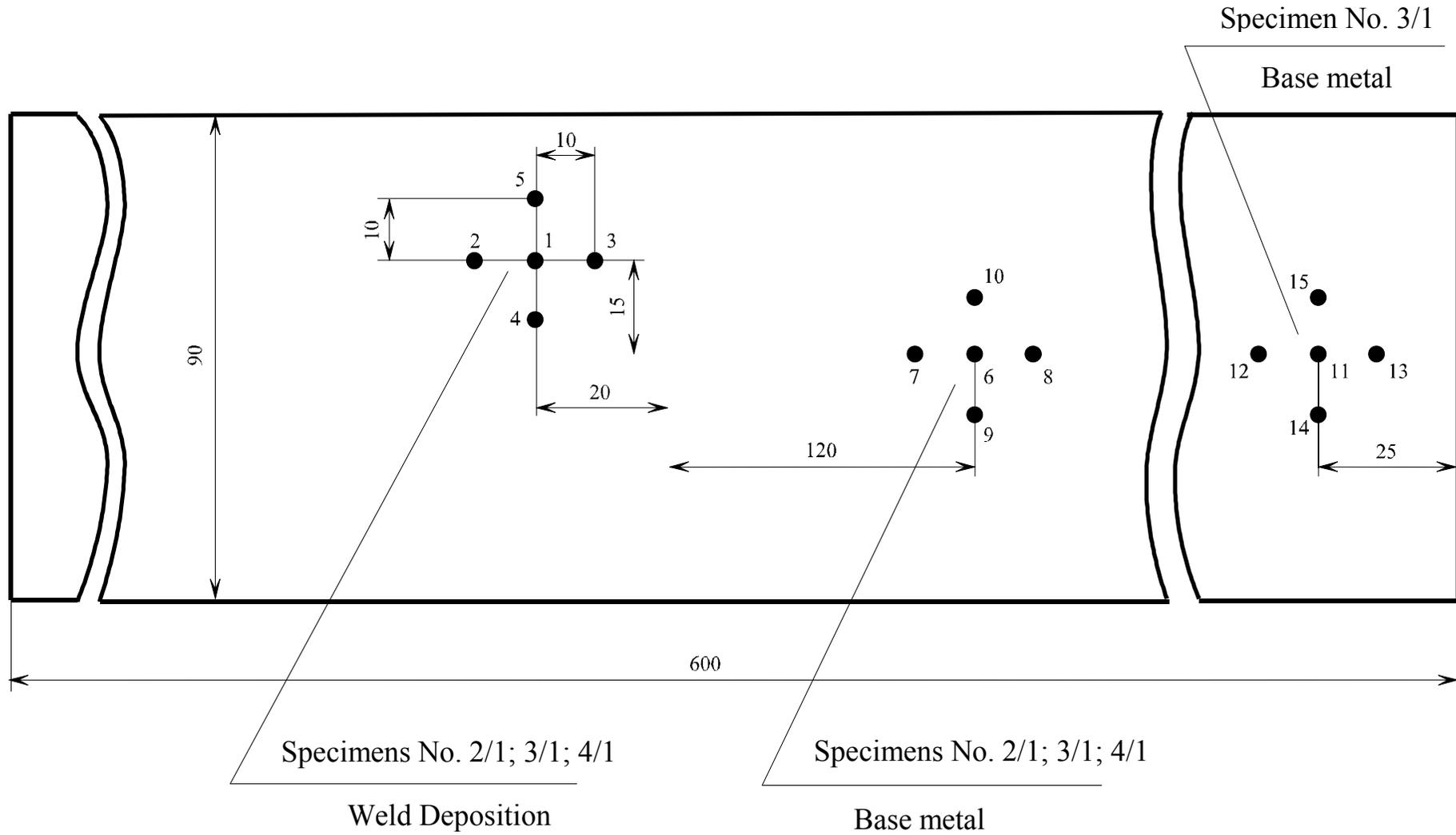
Fig. 10 Diagram of hardness measurement on bronze specimens
