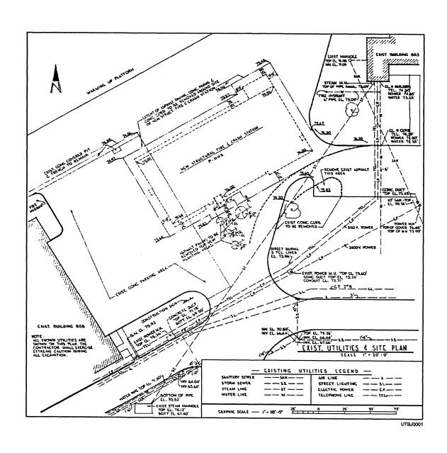
Figure 1-1.—Civil or site plan with existing utilities.
