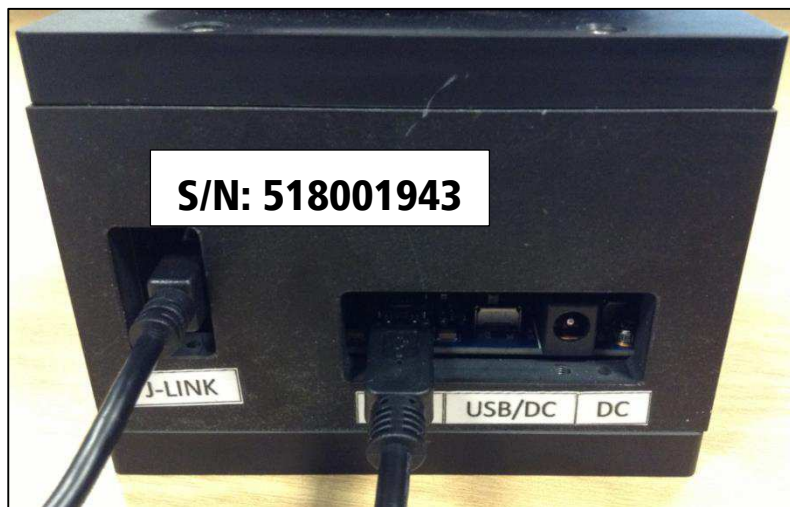
Figure 7: J-LINK cable connecting to programming jig
