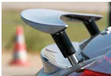
The Cayman S's spoiler deploys at 120 km/h (75 mph).
