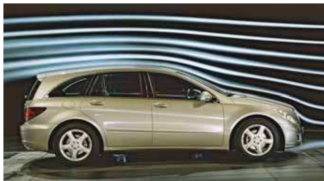
Mercedes-Benz concentrated on the R-Class's aerodynamics to achieve a Cd of 0.31.
