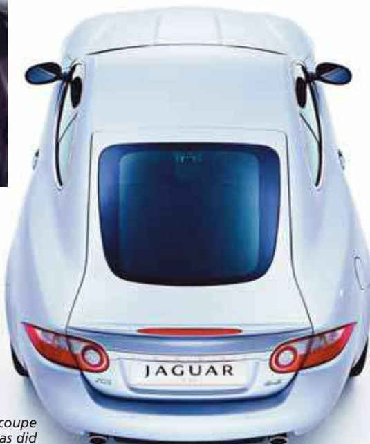
Jaguar's new XK coupe has an aluminum monocoque, for lower mass than the outgoing model, and a side treatment including front wing "power vents" similar to those used by sister company Land Rover for its Range Rover.
