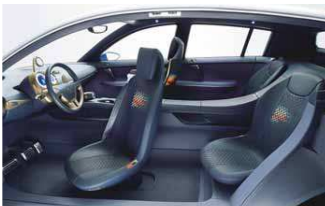
The front seats of the Egeus turn and tilt to aid access and egress.
