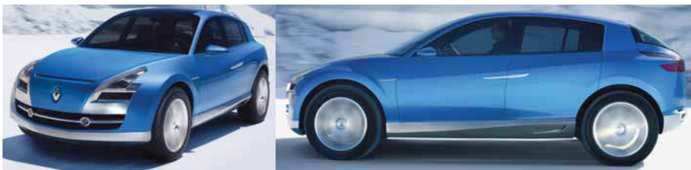
Egeus, Renault's SUV concept, incorporates advanced lighting, backward-opening rear doors, and no B-pillar.
