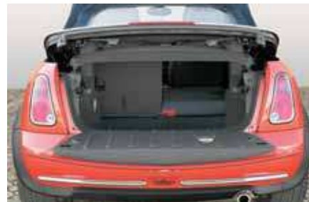
With the roof up, the lower rear edge of the trunk top panel can be unlatched and popped up 35° for access to the trunk and rear seat area.
