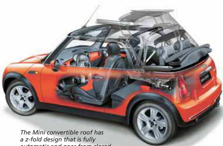
Extra reinforcements for the Mini convertible body structure can be seen in red. The Integrated rear-seat headrests and roll bar are made of high-strength aluminum.
