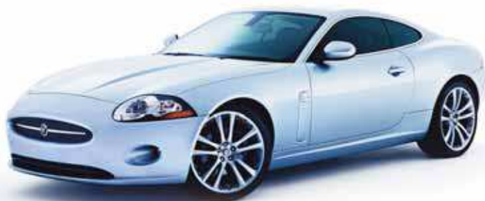
Jaguar's new XK coupe has an aluminum monocoque, for lower mass than the outgoing model, and a side treatment including front wing "power vents" similar to those used by sister company Land Rover for its Range Rover.
