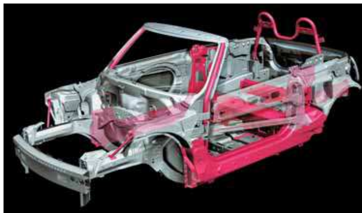
Extra reinforcements for the Mini convertible body structure can be seen in red. The Integrated rear-seat headrests and roll bar are made of high-strength aluminum.
