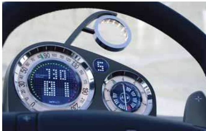
The Egeus' instruments include a speedometer with a warning for recommended speed.
