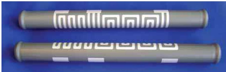
*IRC's Anotherm consists of rugged thick-film resistive elements deposited on tubular anodized aluminum substrate material for a number of applications, including "instant on" cabin heat for diesels, wiper fluid heaters, EGR air intake heaters, fuel pump flow controls, and more.*
