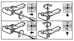
lower the rear sight turn the screw clockwise. When raising the sight the point of impact rises.
