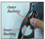
To adjust the hammer tension, remove the grip by loosening the single screw on the bottom of the grip and pulling it free from the frame. The adjustment knob is in the frame. Use a small flat bladed screw driver to hold the inner bushing and turn the outer bushing to adjust. Turn clockwise to loosen the tension and counter-clockwise to tighten. The tension can be checked by verifying that the firearm is unloaded, pointing the muzzle in a safe direction and 'dry-firing' the revolver.
