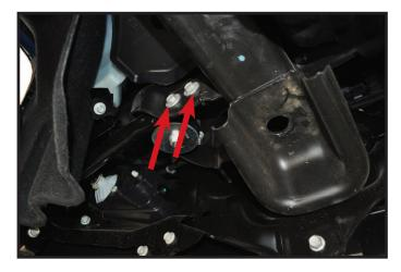
**4.** Remove two bolts from bumper side mount on out side of frame on each side of truck.
