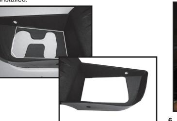
**3.** On GMC Yukon, cut the top portion of the tow hook opening as shown in pictures above. Trim as needed (Plastic cover was removed for viewing purposes). SKIP TO STEP 8.
