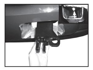
8. Slide base plate pod into frame, and insert previously removed tow hook nut and bolt. **NOTE:** If bolt shown by arrow does not allow baseplate to slide in frame remove point to bolt with saw. **NOTE:** chain anchor hole is to the outside of the vehicle.
