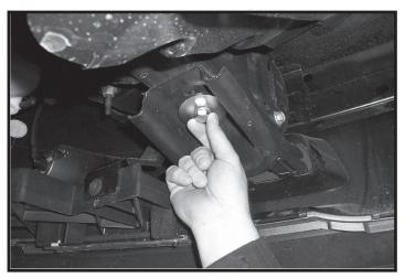
**9.** Install supplied 1/2" x 2" hex bolt, 1/2" lock washer, 1/2" frame washer, and tighten all bolts.
