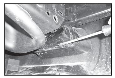
**2.** Remove tow hook plastic filler panels by releasing clips on filler panel from the back side of fascia. These will not be reinstalled.
