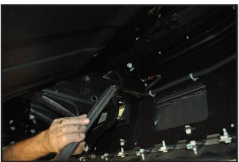
**6.** On the drivers side only take a bar and hammer the top portion of bracket up to allow room for front tow hook removal.
