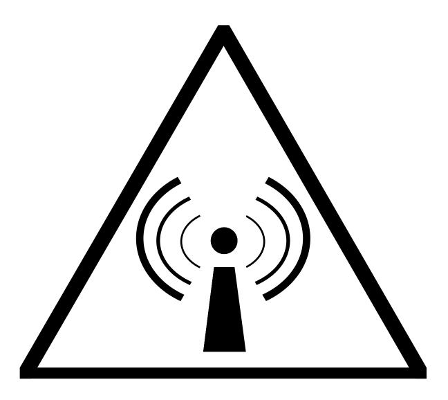
The warning symbol for identifying incident-electromagnetic energy consists of a black wave front radiating from a stylized point-source antenna on a white background. This symbol may be used as a part of safety signs that conform with danger caution, and notice as specified in ANSI Z535.2-1991.
