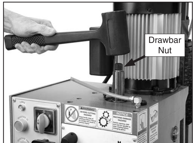
Figure 14. Unseating the arbor/cutter.
