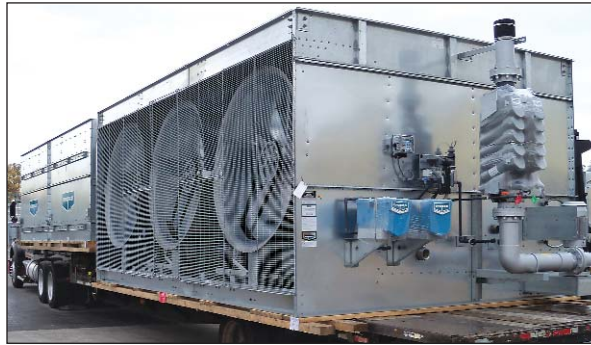
Evaporative Condenser Birmingham, AL USA
