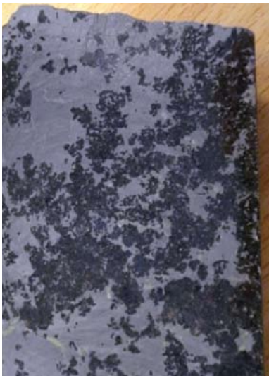
▲ Core hole FRDH001. Massive-blebby Sulphides in FRDH001 at 41.7m downhole
