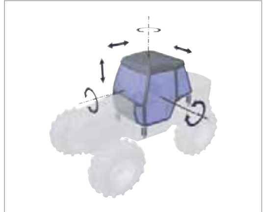
Fig. 4 Movement possibilities of the cabin
