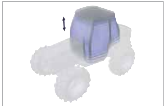
Fig. 5 Vertical vibrations of the cabin before optimisation
