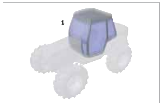
Fig. 6 Vertical vibrations of the cabin after optimisation
