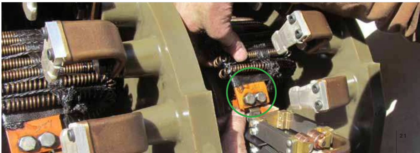
FIGURE 9A: LOCATION OF MEASURED RESISTANCE VALVE
