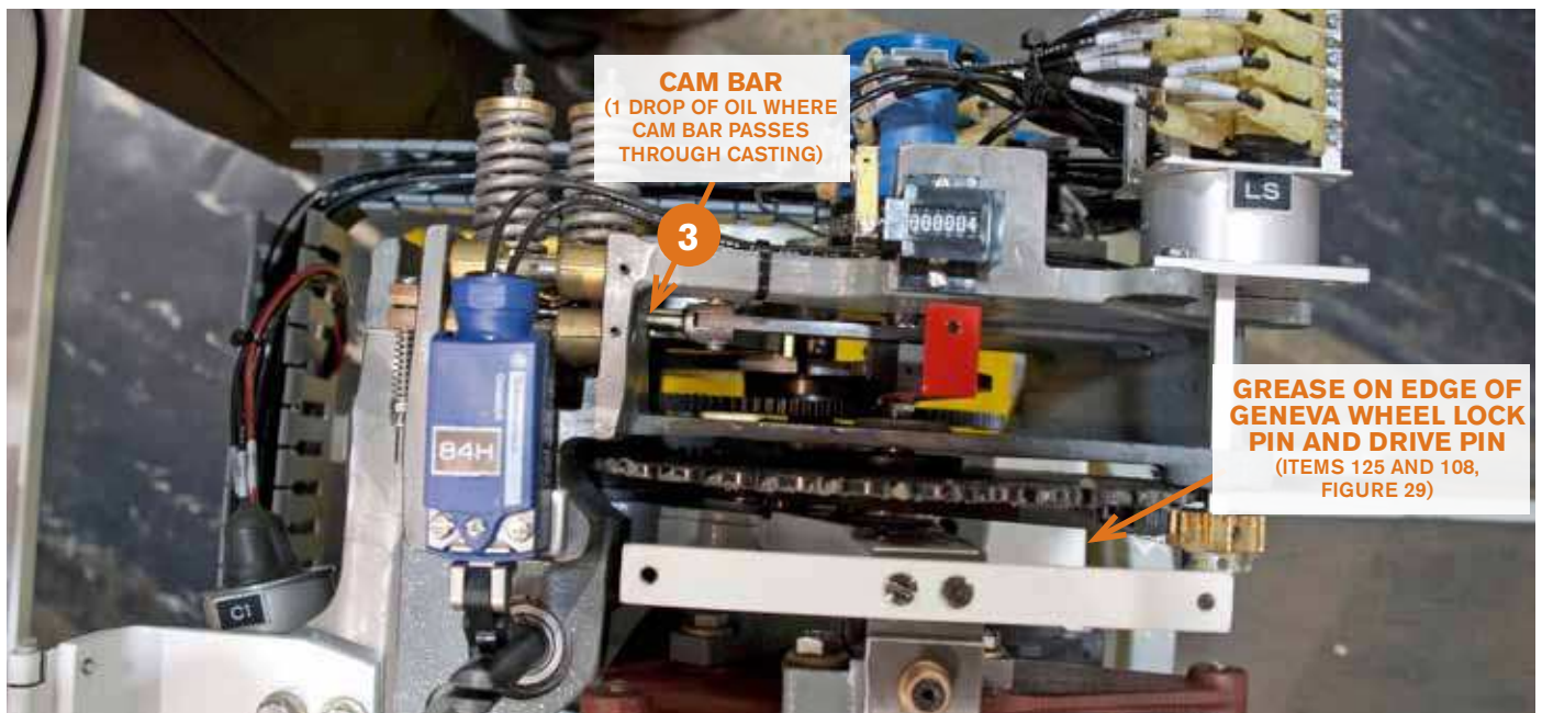
FIGURE 34: OILING OF CAM BAR, GREASING GENEVA WHEEL
