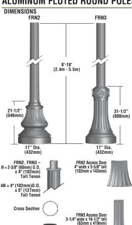
**POLE SHAFT** - The pole shaft is either spun or extruded from 6000 series alloy aluminum. Tenon N option is 2-3/8" O.D. x 4" tall. Tenon 4N option is 4" O.D. x 5" tall. Aluminum 16 flat fluted round pole shafts with decorative base are 4", 5" and 6" in diameter. Poles have a cast ring between shaft and tenon.
