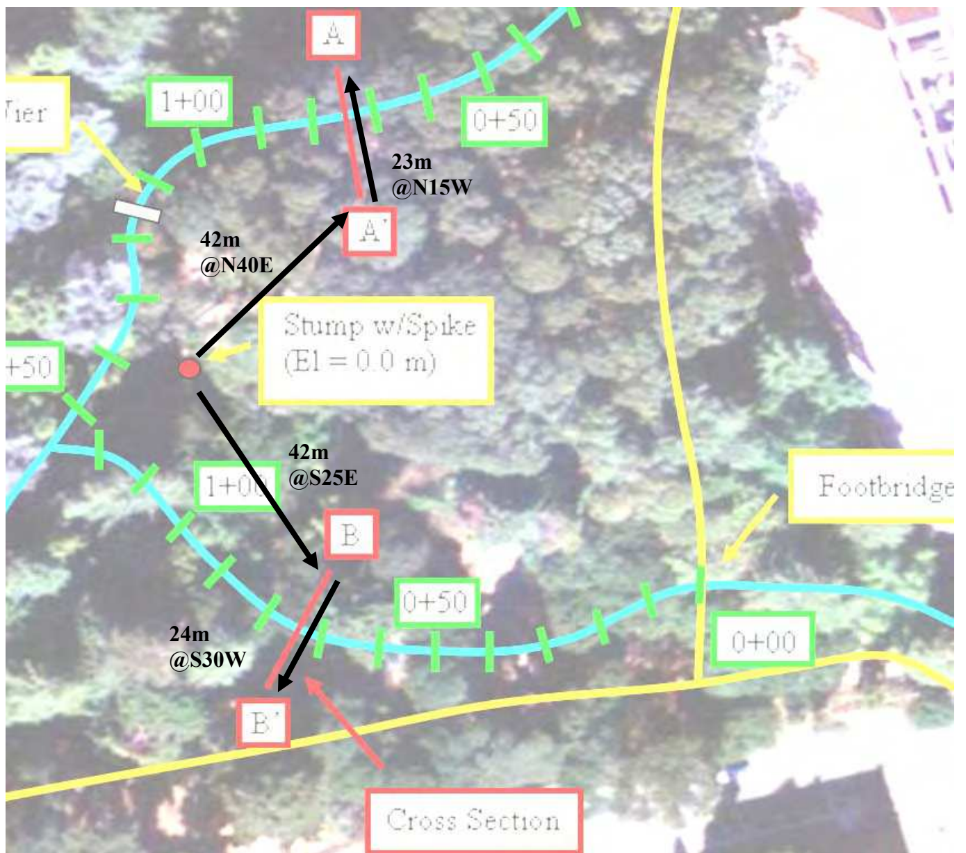
Figure 11 – Noting locations of cross-sections with distance and bearing measurements made using a tape and hand compass.
