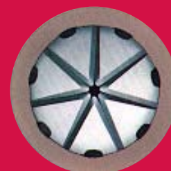
Variable Inlet Guide Vanes – Variable inlet guide vanes can offer power savings of up to 9%. Inlet vanes impart a whirling motion to the inlet air flow in the same direction as the impeller operation, reducing the work input. Net power savings at reduced flow or on days colder than the design temperature. Inlet vanes are positioned close to the impeller to achieve maximum benefit.
