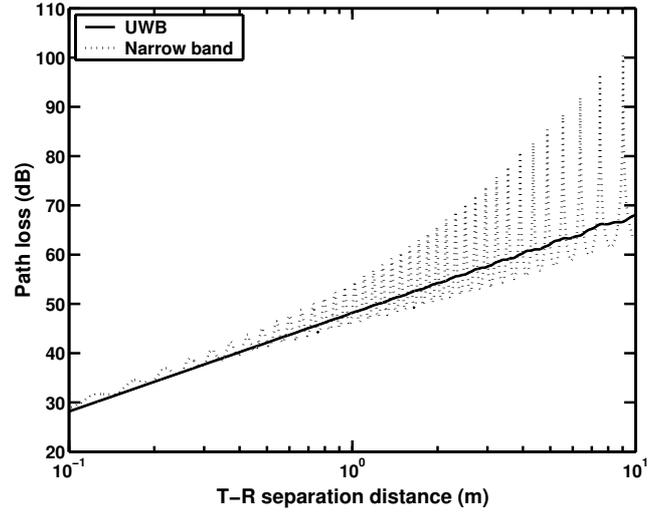
Fig. 3. UWB path loss for the 1.00 m antenna heights along T-R separation distance from 0.1 to 1 m compared with narrow band path loss.
