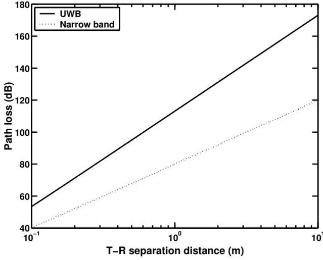
Fig. 5. UWB path loss for the 0.01 m antenna heights along T-R separation distance from 0.1 to 1 m compared with narrow band path loss.
