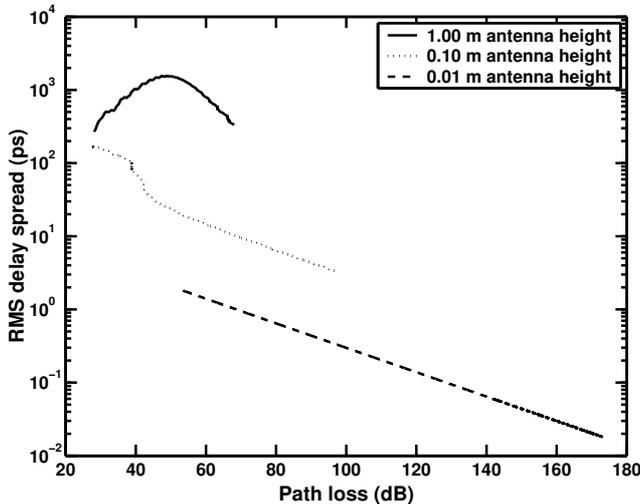
Fig. 6. RMS delay spread versus path loss for 1.00, 0.10 and 0.01 antenna heights.
