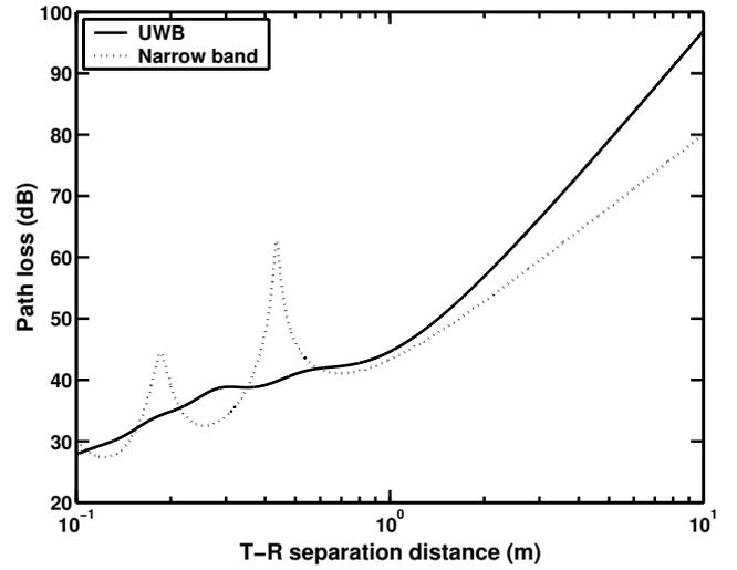
Fig. 4. UWB path loss for the 0.10 m antenna heights along T-R separation distance from 0.1 to 1 m compared with narrow band path loss.
