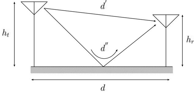
Fig. 1. Ground reflection model.
