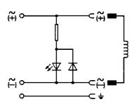
12 V DC/24 V AC/DC 100-120 V AC/DC 200-240 V AC/DC polarity!
