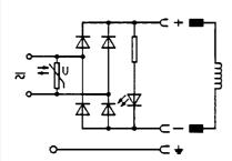
12- 24 V AC/DC 100-120 V AC/DC 200-240 V AC/DC Order-No.: 008 354 Q Order-No.: 008 355 R Order-No.: 008 356 J With rectifier and varistor
