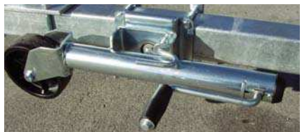
Fig 4: Swing jack in traveling position.
