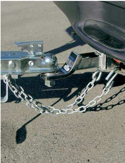
Fig 3: Proper attachment of the safety chains is essential to trailer safety. Note how the safety chains are crisscrossed.
