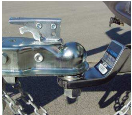
Fig. 2: Coupler on ball with latch in proper lock position.
