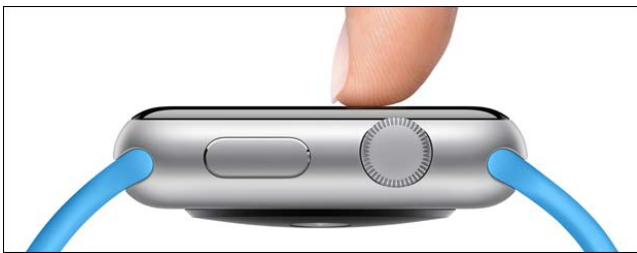
Force-sensitive Retina display on the top, Taptic sensors on the bottom.
