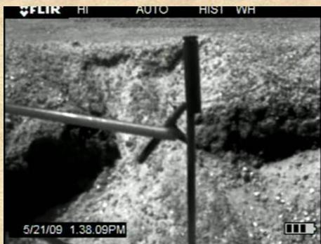
Tank Gas Pipe Routed Close to Flare (IR Video)
