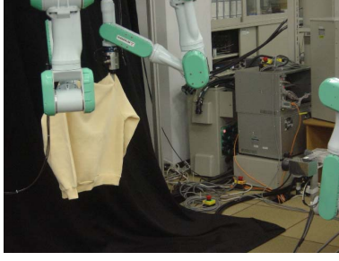
Figure 1: System consisting two manipulators and stereo cameras
