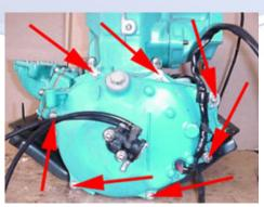
5.3 (Below) Remove the six 12mm nuts securing the exhaust manifold to the engine and remove the manifold.
