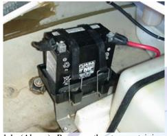
1.1 (Above) Remove the two retaining straps, disconnect the battery and remove it from the hull. Disconnect the negative (black) cable first, then the positive (red).
