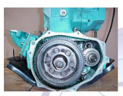
5.6 (Below) Stuff a rag into an open exhaust port. This will prevent the engine from turning over while removing the flywheel and PTO coupler.
