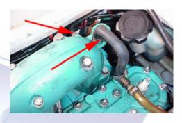
3.2 (Below) Remove the four 14mm bolts securing the exhaust pipe to the manifold, and the case-dump handle mount nut (handle removed for better view). Do not disturb the rubber stinger to head pipe joint. Replacement joint parts will often be necessary if this part is removed.
