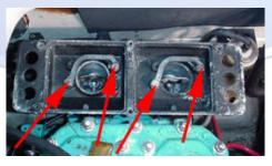
2.5 (Below) Disconnect the throttle and choke cable ends from the carbs.
