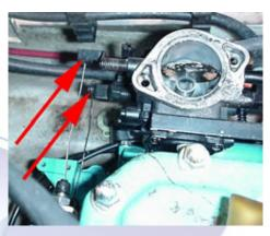
2.6 (Above) Loosen the gas tank cap to relieve pressure. Be sure the fuel switch is turned to the "OFF" position, and be aware of any fuel that may spill from the hoses. Make sure the hull is clear of any gasoline fumes before continuing work, especially with power tools. Disconnect the pulse line, fuel in and fuel out lines from the carbs.
