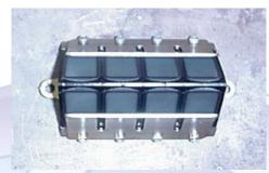
2.11 (Below) Look at each petal-to-cage surface and check for gap. If a gap of more than 0.015" is present, replace the petals.
