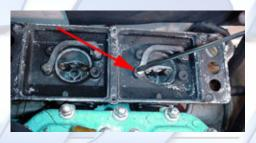
2.4 (Above) Remove the four 10mm bolts securing the flame arrestor base and carbs to the manifold and remove it.
