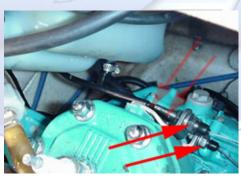
4.3 (Below) Remove the starter positive and ground cables with a 10mm socket.
