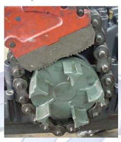
5.8 (Below) Remove the four bottom plate 14mm bolts and remove the plate.
