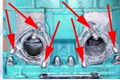
5.4 (Above) Remove the six 8mm studs with a stud socket.
