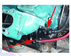
4.4 (Below) Remove the two 10mm bolts from the wiring cover on the electrical box, exposing the wiring harnesses. Disconnect the harnesses.
