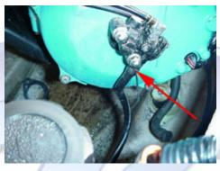
4.2 (Below) Remove the throttle and choke cables from the support bracket, and remove the two 10mm bolts securing the bracket to the engine – remove it.
