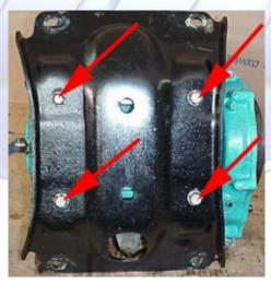
5.9 (Below) Remove the two 12mm bolts securing the case dump mechanism to the engine and remove it.
