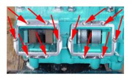
2.10 (Below) Inspect each reed assembly for damage and wear. Look at each reed petal and inspect the edges for signs of cracking, chipping or any missing parts. If any damage is present, replace the petals.
