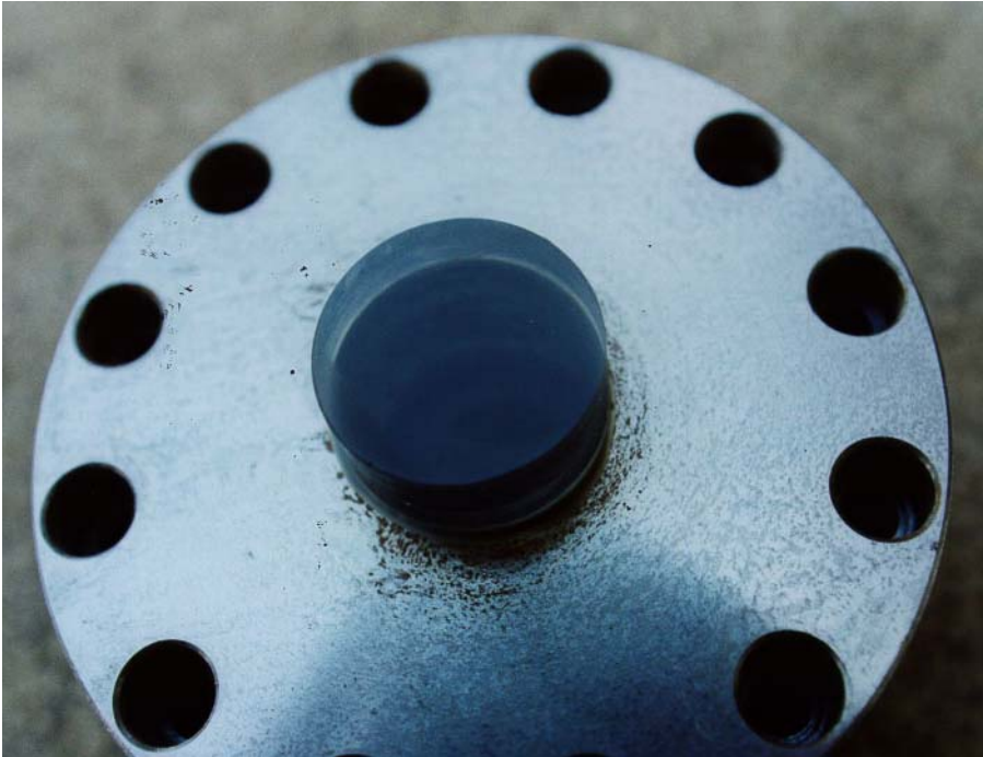
Figure 2.7 Close-up photograph of glass mounted in steel chuck
