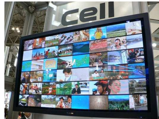
Simultaneous decoding of 48 MPEG-2 streams
