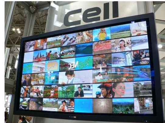
Simultaneous decoding of 48 MPEG-2 streams
