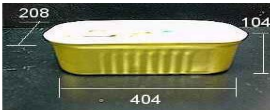
Figure 18 – Measurement of a Low-Profile Container
