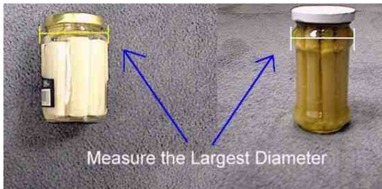
Figure 13 – Measurement of an Unusual Shape Cylindrical Container.
