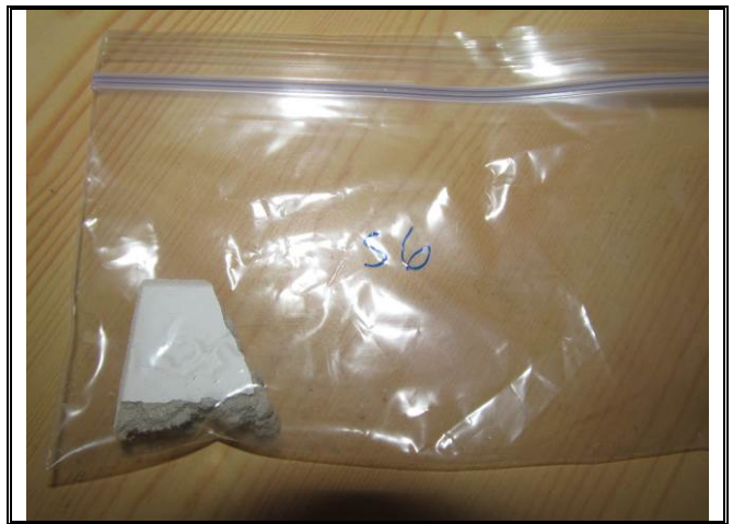
Photograph No. 017: Sample 6 - Drop ceiling tile
