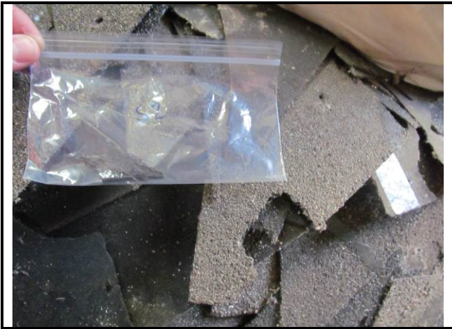
Photograph No. 008: Sample 2 – Roofing asphalt, paper and tar
