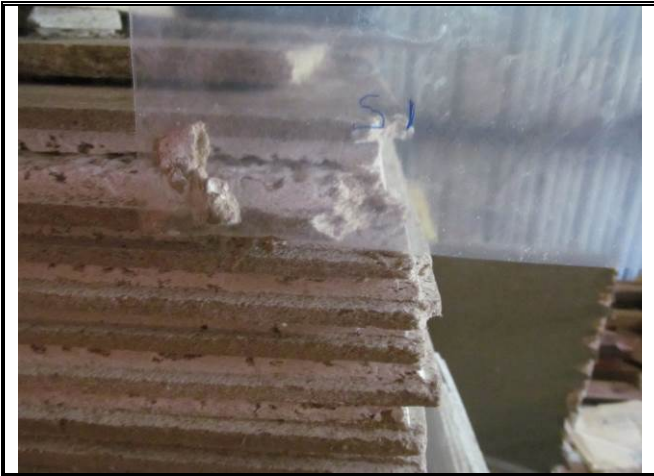
Photograph No. 007: Sample 1 – Drop Ceiling tile 12x12
