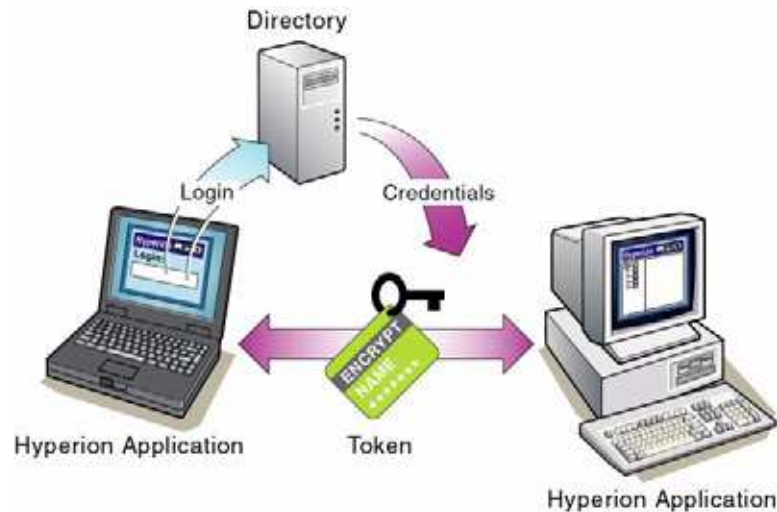
Figure 4 Authentication to External Provider Enables Remote Authentication to Reach Multiple Applications
