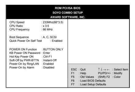
After the hardware installation is complete, turn the power switch on, then press the <DEL> key during the system diagnostic checks to enter the Award BIOS Setup program. The CMOS SETUP UTILITY will display on screen. Then, select the [SOYO COMBO SETUP] option from the main menu and press the <Enter> key.
