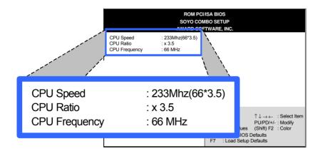
Available [CPU Speed] settings on your SY-6IEB Mainboard are detailed in the following table. If you set this field to [Manual], you are then required to fill in the next two consecutive fields: (1) the CPU Ratio, and (2) the CPU Frequency.
