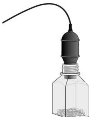
Figure 1. Vernier O 2 gas sensor probe and reaction chamber ready to collect data.
