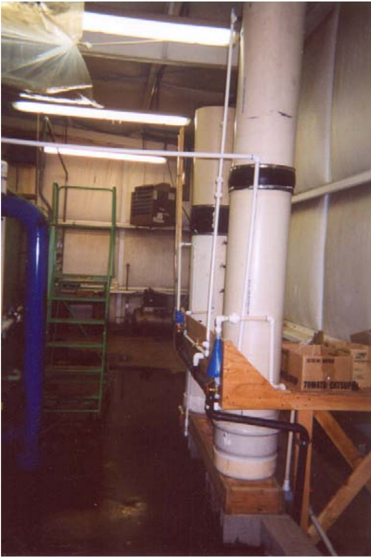
Figure 3-2. Typical Slow Sand Pilot Apparatus
