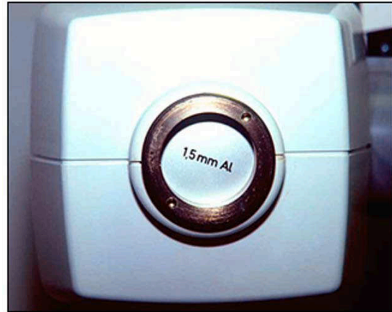
Figure 5. 1.5 mm of Aluminum Filtration
