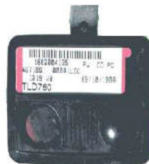
Figure 14 Personnel Monitoring Device
