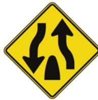
Divided Highway Ends
