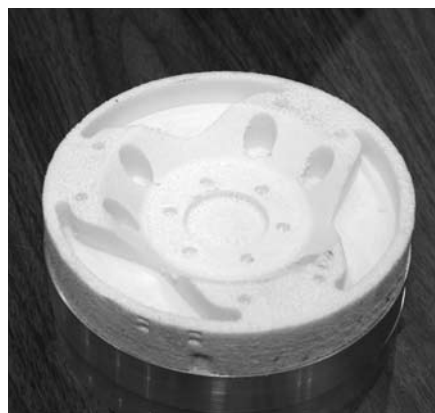
Brake Rotor hat - machined in foam prior to committing to aluminum.
