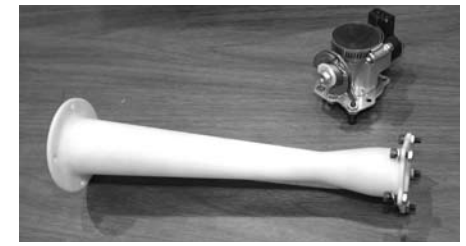
The Rapid Prototype derived air intake with 20mm restriction.
