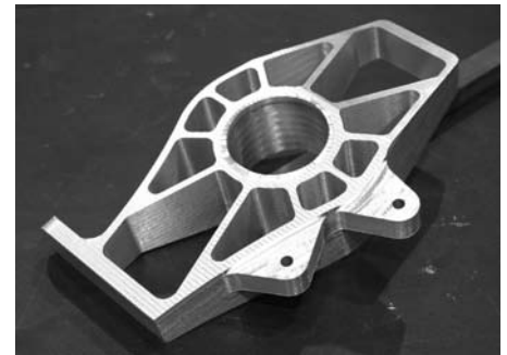
Uprights for the 2007 car were machined from 7075 Aluminum.
