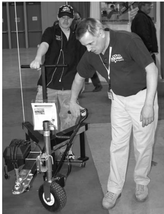
Bill Bonnow takes a virtual trailer for a drive with a new electric nose wheel that allows one person to easily move a large trailer.
