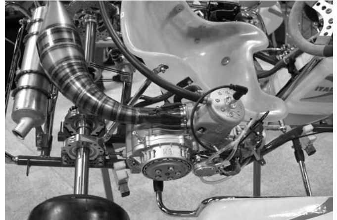
The business end of a modern water cooled shifter Kart. On board starter makes it a one person show.
