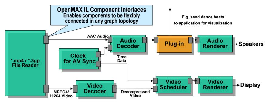
Example: MPEG-4 video synchronized with AAC audio decode
