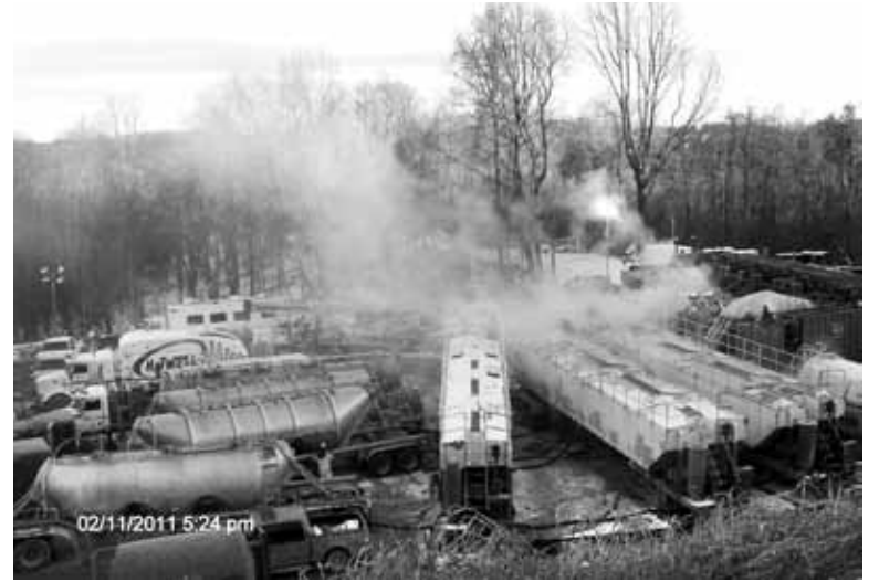
Fine silica dust released almost constantly into the air during the fracking of a Chesapeake well in Wetzel County. It can cause silicosis. PHOTO/BILL HUGHES, WETZEL COUNTY ACTION GROUP
