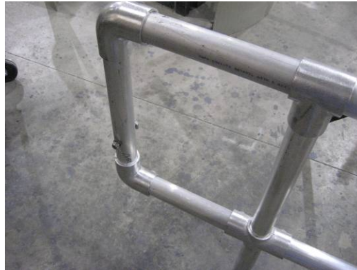
Match drill the ladder to the handrail.
