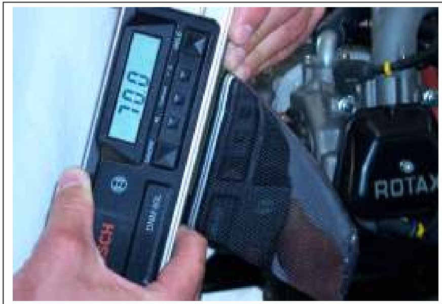
Figure 58 Setting the Blade to 70 Degrees at 24 inches
