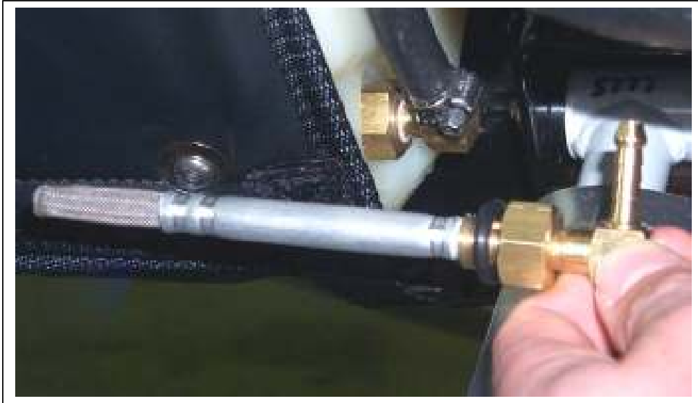
Figure 29 Finger Filter, as installed, as well as the unit prior installation.
