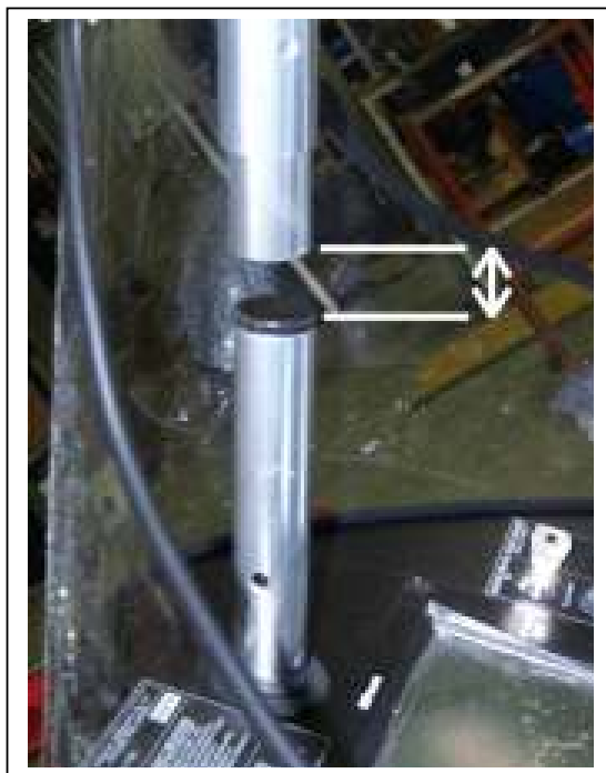
Figure 7 Front Mast to Mast Brace Check
