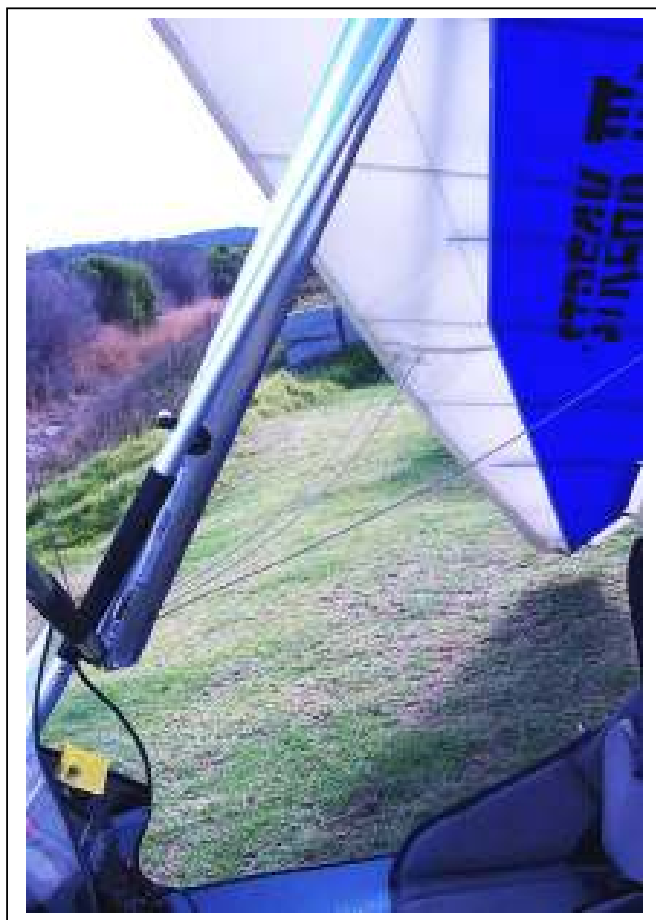
Figure 14 Securing of Base Bar With Bungee
