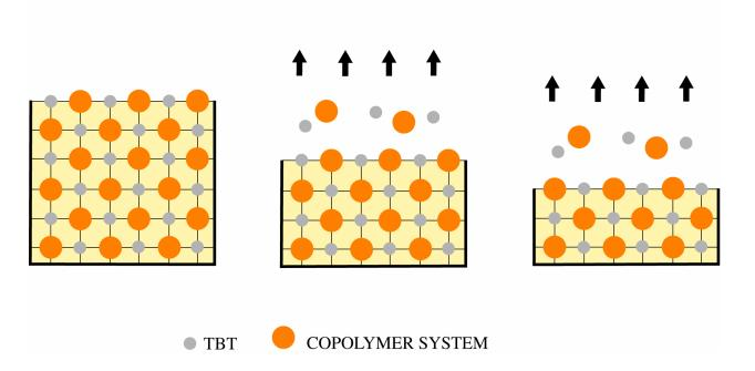
Sea water hydrolyses the TBT copolymer bond and the TBT biocide and copolymer resin is slowly released at a controlled rate. Uniform anti-fouling performance is achieved throughout the lifetime of the paint. *Source*: CEFIC.
