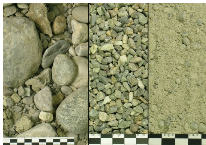
Figure 4: Crystalline-rich, sandy gravel before preparation (left picture), before (middle picture) and after (right picture) LCPC test. Scale: 1 black bar equals 1 cm (1 pitch line equals 1 mm).
