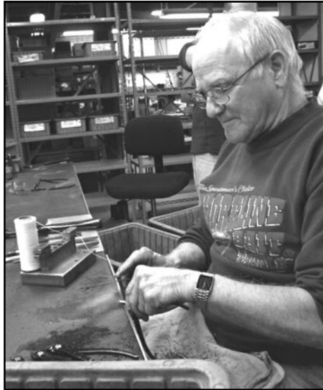
At far left, Doug Cordner grinds and sizes the two halves of the cutting tools. Ralph Bolduc files a cutter, at left. This process is done by hand on every tool manufactured by Xuron. Above, Tina Brown packages tools for shipping.
