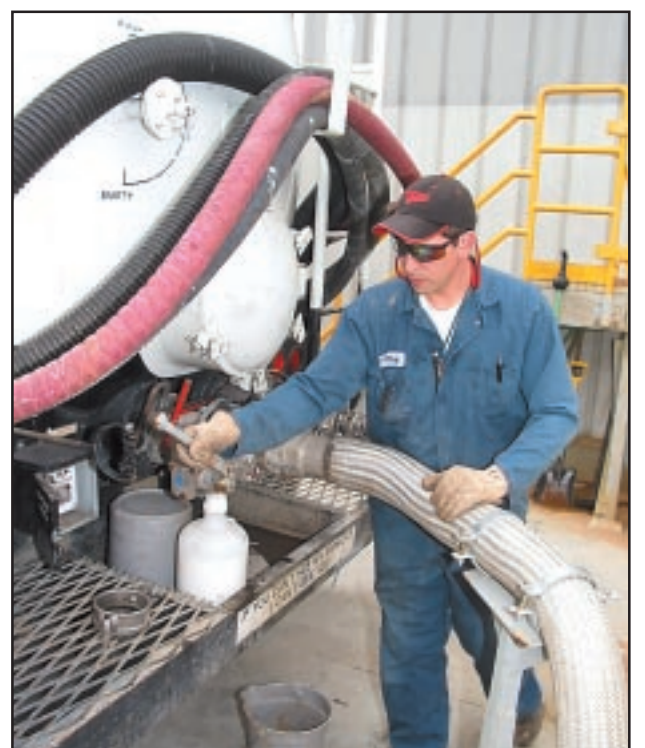
Chad Kiehn transfers waste water from the Renton plant to the 4-83 building treatment center to remove chemicals so the water can be discharged into the sewer system.
