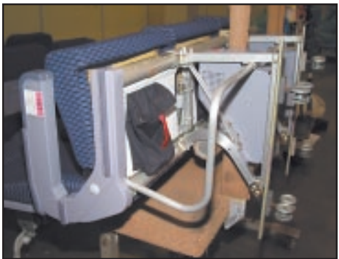
Above: Members suggested installing life vests while the seats are tipped, which eliminated hours from the job and kept the work in-house.
