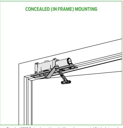
The concealed 5010 Series is a heavy duty closer designed for institutional, high traffic, or other applications exposed to weather or abuse. The double lever arm provides superior door control and a choice of finishes, cylinder functions, and arm functions that meet virtually all architectural requirements.
