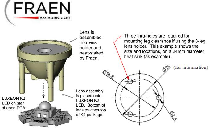
Dimensions tolerance is +/-0.2mm
