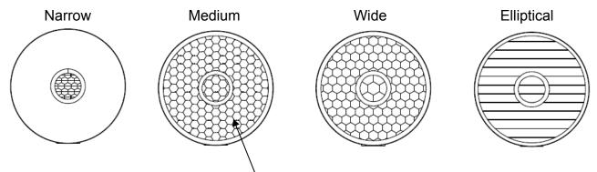
The medium beam lens has a light texture on the micro-lenses.
