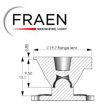
Dimensions of lens on K2 LED (lens shown without lens holder):
