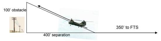
The CH 46 is 85' in length, 51' width, 17' height. The CH 47 is 99' in length, 60' width, 19' height.
