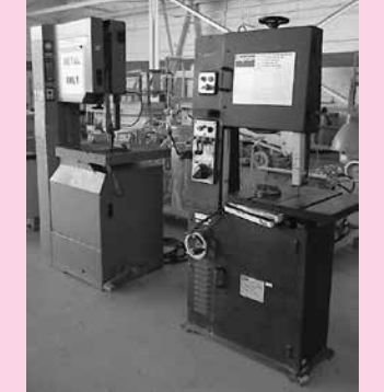
Dayton Mdl 4TK02 18" Band Saw w/ Blade Welder, 18" Throat, 20" x 22" Tilt Table Rockwell-Delta Series 28-3X5 Band Saw, 20" Throat, 24" x 24" Tilt Table
