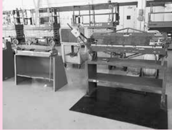
Jet Mdl BP-1648 48" Sheet Metal Finger Brake, 16 Gauge Capacity Berkroy Mdl B-936 36" Sheet Metal Finger Brake
