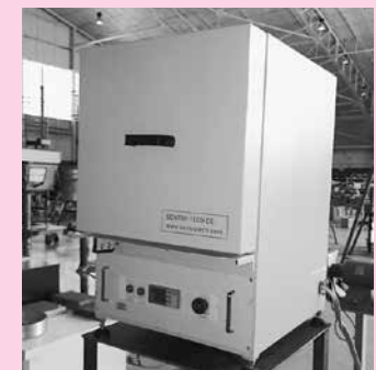
Sentro Tech ST-1200-7812-AG High Temp Heat Treat Furnace, 1,200° C Max Temp, Chamber Size 7" x 8" x 12", Digital Temp Controller
