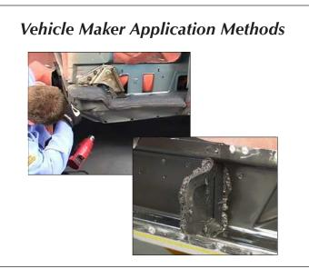
During vehicle assembly, foam may be installed in different ways. These include:
