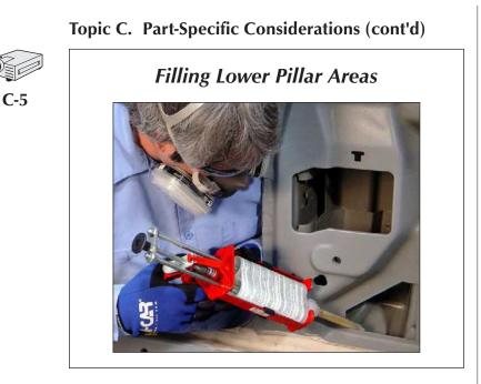
When filling lower pillar areas with foam, follow the vehicle maker's recommendations. When installing foam in lower pillars:
