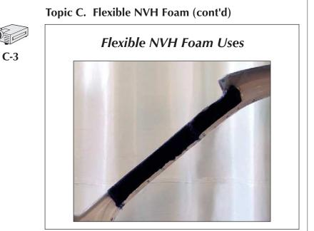
Some uses for flexible foam include controlling panel flutter, absorbing and controlling sound, and blocking air movement. Another use for flexible foam includes filling large voids.
