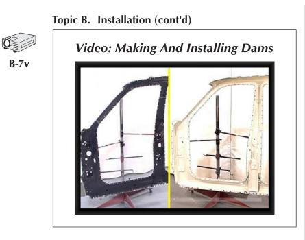
This video shows ways of making and installing dams to retain foam.
