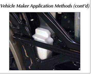
Set-in position foam consists of two types. The first type is a solid material that is set into position and clipped or bolted to the door shell assembly. The other type of set-in position foam is flexible foam block. These blocks are typically encased in a plastic bag so they do not absorb water. Depending on the vehicle maker's design, these blocks may be located anywhere on the vehicle. Flexible foam parts may also be called stuffers. Instructor Information
