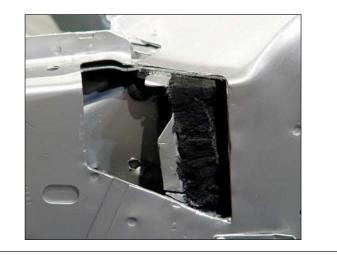
Chemical-cure foams used during the vehicle assembly process:
