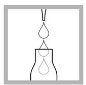
**10.** Pipet into the cooled cuvette: **0.2 mL Reagent B**. Close Reagent B **immediately** after use.
