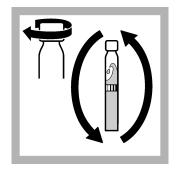
**12.** Close the cuvette and invert a few times until the freeze-dried contents are **completely dissolved**.
