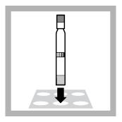
6. Heat in the thermostat. HT 200 S: in the standard program HT for 15 minutes. Thermostat:
