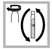
**4.** Close the cuvette and invert a few times until the freeze-dried contents are **completely dissolved**.
