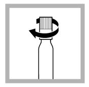
**4.** Immediately screw the DosiCap Zip back on tight; fluting at the top.
