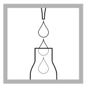
2. Pipet 0.2 mL Reagent B. Close Reagent B immediately after use.
